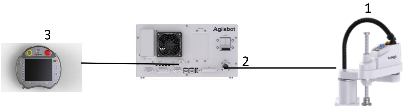
1- Robot body 2 - Controller 3 - Teach pendant
